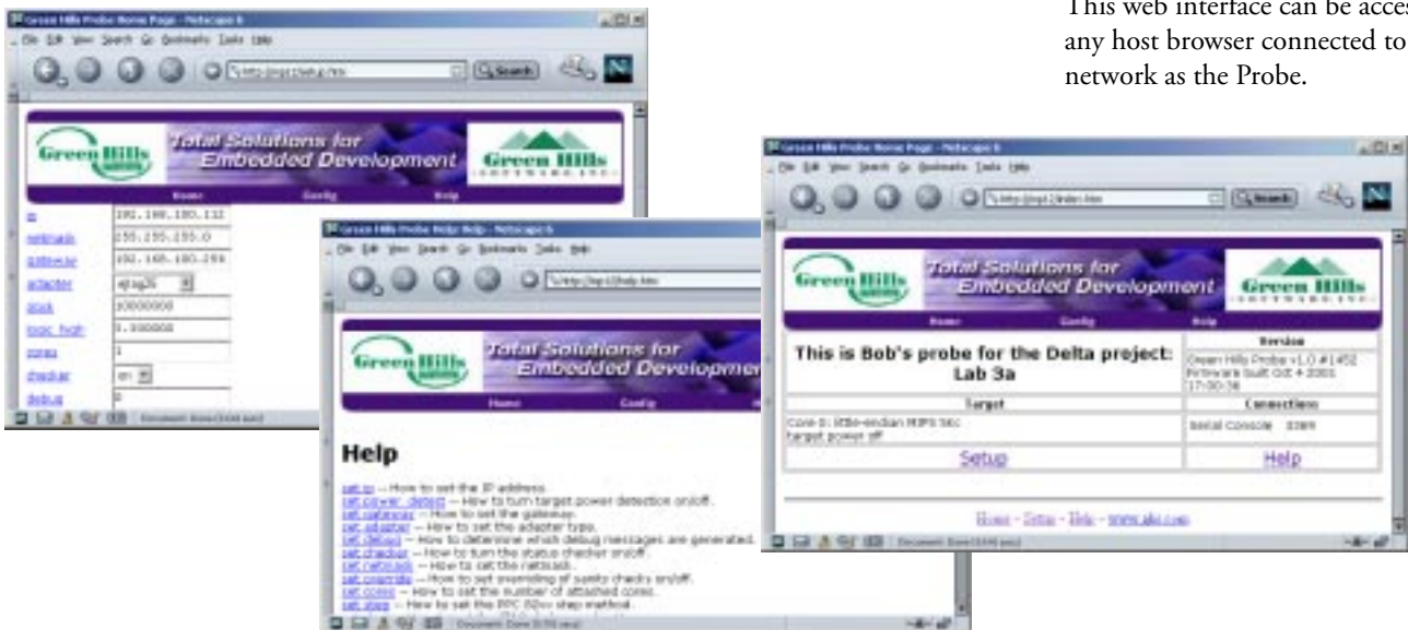
The Probe's web interface is accessible through an Ethernet connection and viewable with most any web browser. With it, you can configure debugging options as well as display information about the Probe, connection, and target.
